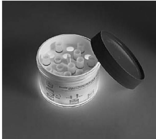
**Figure 6.6** A photograph of the Nalgene® Mr. Frosty. This device should approximate a freezing rate of  $1^{\circ}\text{C}/\text{minute}$  when placed in a minus  $70^{\circ}\text{C}$  freezer. Notice the cryovials placed in the insulated container
