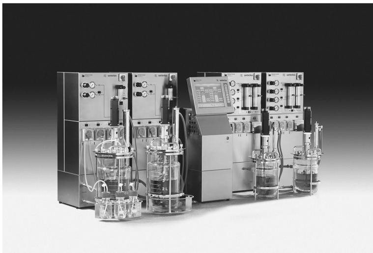
**Figure 5.1** Typical bench top cell culture bioreactors. Note the height of condenser, which significantly increases overall height and thus determines type of autoclave required. (Reproduced by permission of Sartorius Biotechnology Ltd)
