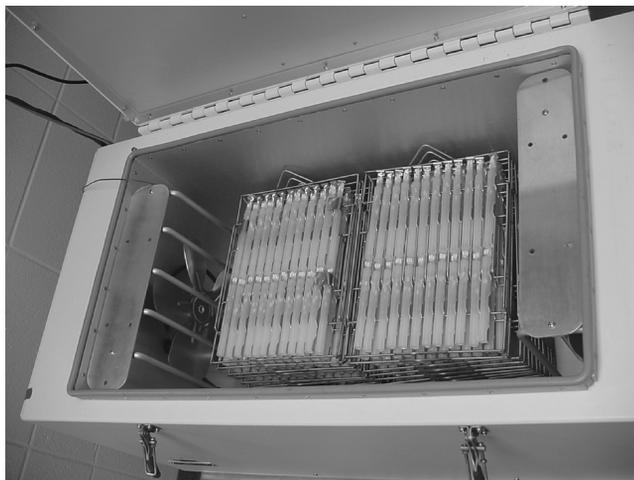
**Figure 6.4** A photograph of a controlled-rate freezer containing racks of straws ready for freezing. Notice the large capacity cooling fan on the left side – there are two fans, one on each end to facilitate uniform cooling
