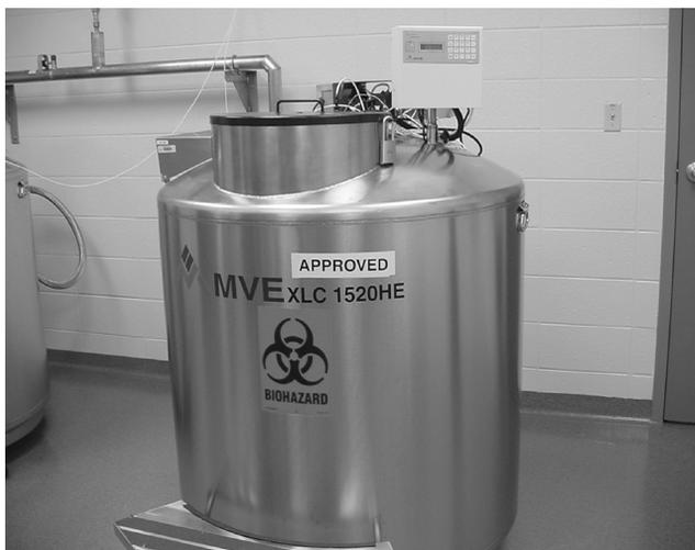
**Figure 6.7** Photograph of a high efficiency, automatic-fill cryogen. Notice the vacuum-jacketed piping for delivery of LN<sub>2</sub>
