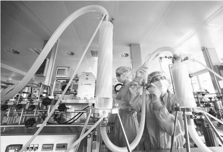
**Figure 5.5** Example of Midicap filters being used in production (Reproduced by permission of Sartorius Biotechnology Ltd)
