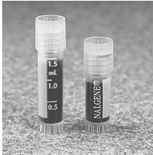
**Figure 6.1** A photograph of polypropylene screw-cap cryovials. Notice the external threads that facilitate sterile technique and the thin internal gasket for sealing cap. Remember, these can be used in LN<sub>2</sub> vapor phase only
