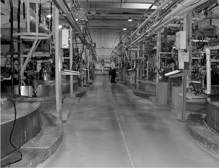
**Figure 8.14** Photograph of production fermentation facility used for natural product fermentations
