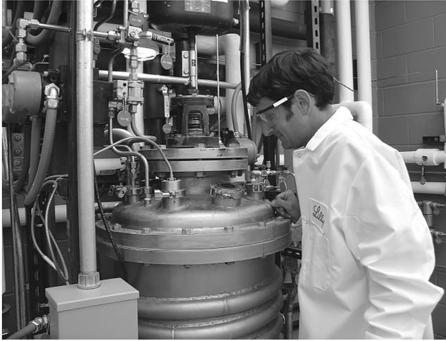
**Figure 8.11** Photograph of scaled down geometric fermentation vessels used for fermenting *Streptomyces* spp (Eli Lilly and Company, Inc)
