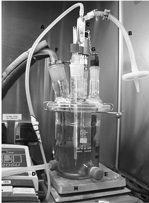
**Figure 12.4** A small experimental chemostat (500-mL working volume). A: medium feed (from peristaltic pump); B: air supply via on-line filter (to be collected to supply); C: medium break; D: effluent line carrying air exhaust and culture from overflow; E: port for sampling by means of hypodermic needle and syringe; F: water supply and return for constant temperature coil; G: pH and oxygen electrodes (not connected); H: magnetic stirrer bed
