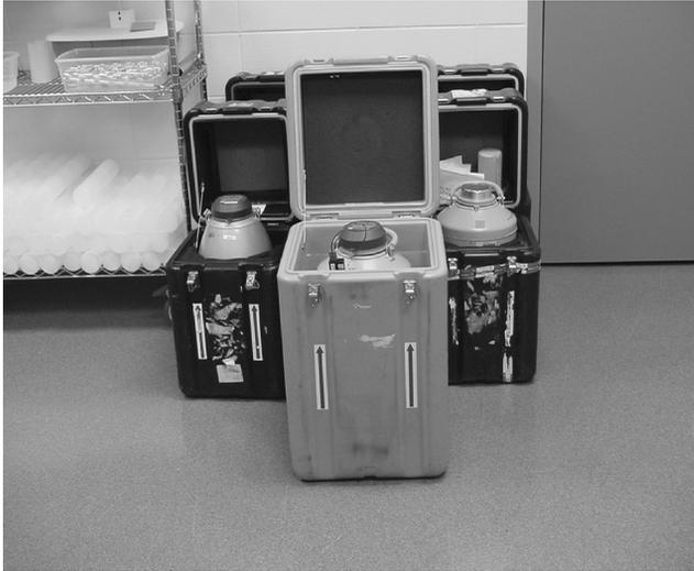
**Figure 6.9** A photograph of LN<sub>2</sub> vapor phase Dewar flasks secured in their shipping cases
